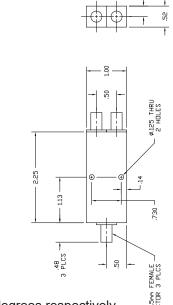
Amplitude and phase tracking are the ratio of one output to the other in dB or degrees respectively. Input power rating is 10 watts with 2:1 load VSWR's.
