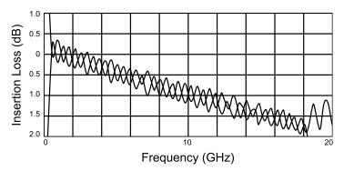
Figure 2: Insertion Loss of Model 4010180 Hybrid
