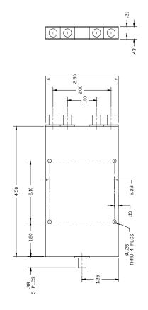
Amplitude and Phase Tracking are the ratio of one output to the other in dB or degrees respectively. Input Power Rating is 10 watts with 2:1 load VSWR's.
