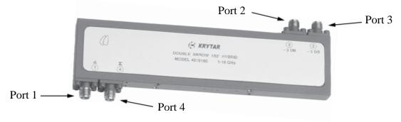
When a signal is applied to port 1, the output signal will appear on ports 2 and 3. Ports 2 and 3 are 180 degrees out of phase with each other.
