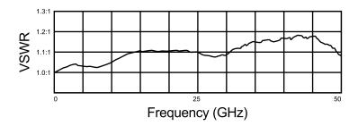
Figure 2: VSWR vs Frequency, Krytar T4M Termination
