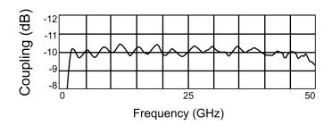
(Figure 1) Coupling characteristics of Krytar Model 102050010
