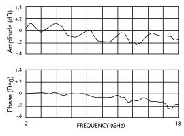
Figure 2: Typical Model 1830 amplitude and phase imbalance.
