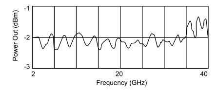
(Figure 1) Frequency Response of Model 202040013 Directional Detector
