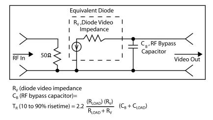
Figure 1: Equivalent Circuit for Krytar Detectors
