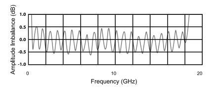
Figure 1: Amplitude Imbalance for Model 4010180 Hybrid
