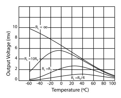
Curves are normalized to  $R_{L}=\infty$  and  $T_{a}=20^{\circ}\text{C}$ ,  $R_{v}$  corresponds to the load that drops the open circuit ouput voltage in half (3dB) at 20°C.
