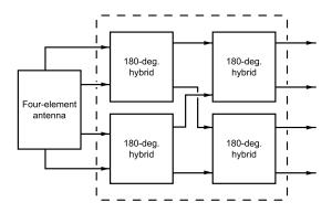
Figure 2: Beam Forming Network
