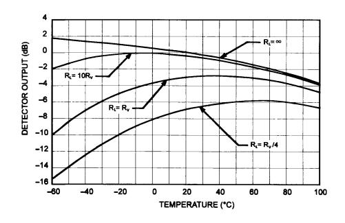
Curves are normalized to  $R_{\perp} = \infty$  and  $T_a = 20^{\circ}$ C,  $R_{\nu}$  corresponds to the load that drops the open circuit ouput voltage in half (3dB) at 20°C.
