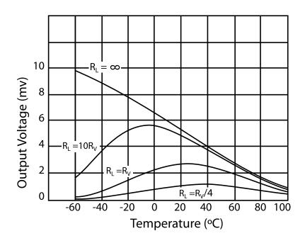
Curves are normalized to  $R_{L}=\infty$  and  $T_{a}=20^{\circ}\text{C}$ ,  $R_{v}$  corresponds to the load that drops the open circuit ouput voltage in half (3dB) at 20°C.
