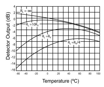
Curves are normalized to  $R_L$ =  $\infty$  and  $T_a$ =20°C.  $R_V$  corresponds to the load that drops the open circuit output voltage in half (3dB) at 20°C.
