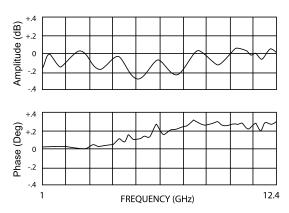
Figure 1: Typical Model 1230 amplitude and phase imbalance
