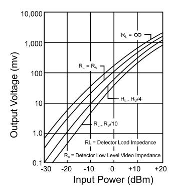
TYPICAL LOW LEVEL (Pin  $\leq$  -20 dBm) OUTPUT RESPONSE vs. TEMPERATURE CURVES FOR VARIOUS R<sub>L</sub>/R<sub>v</sub> RATIOS
