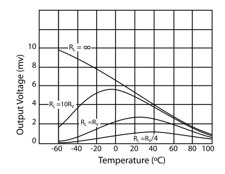
Curves are normalized to  $R_{L} = \infty$  and  $T_{a} = 20^{\circ}$ C,  $R_{v}$  corresponds to the load that drops the open circuit ouput voltage in half (3dB) at 20°C.
