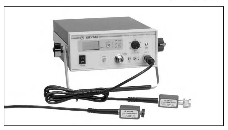
The Krytar Model 9000B is a low cost, high performance CW power meter using a diode based power sensor. The power meter can measure power levels from -39 to +20 dBm and cover frequencies from 100 kHz to 40 GHz. With bench and field service applications in mind, the power meter was designed to be completely portable. The power meter can be used for swept measurement.
